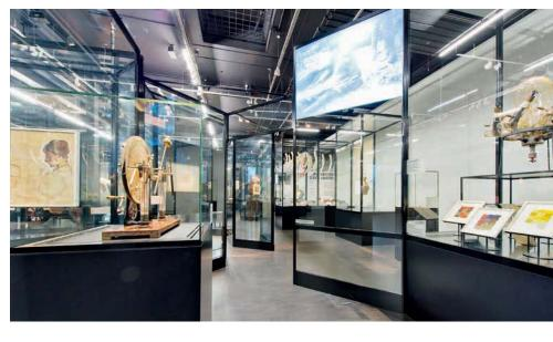
der-coated SYMA-SYSTEM 30, black painted MDF board and 6mm laminated safety glass with reflective foil were used. A major advantage here is that the majority of the system can be reused for the next exhibition.
